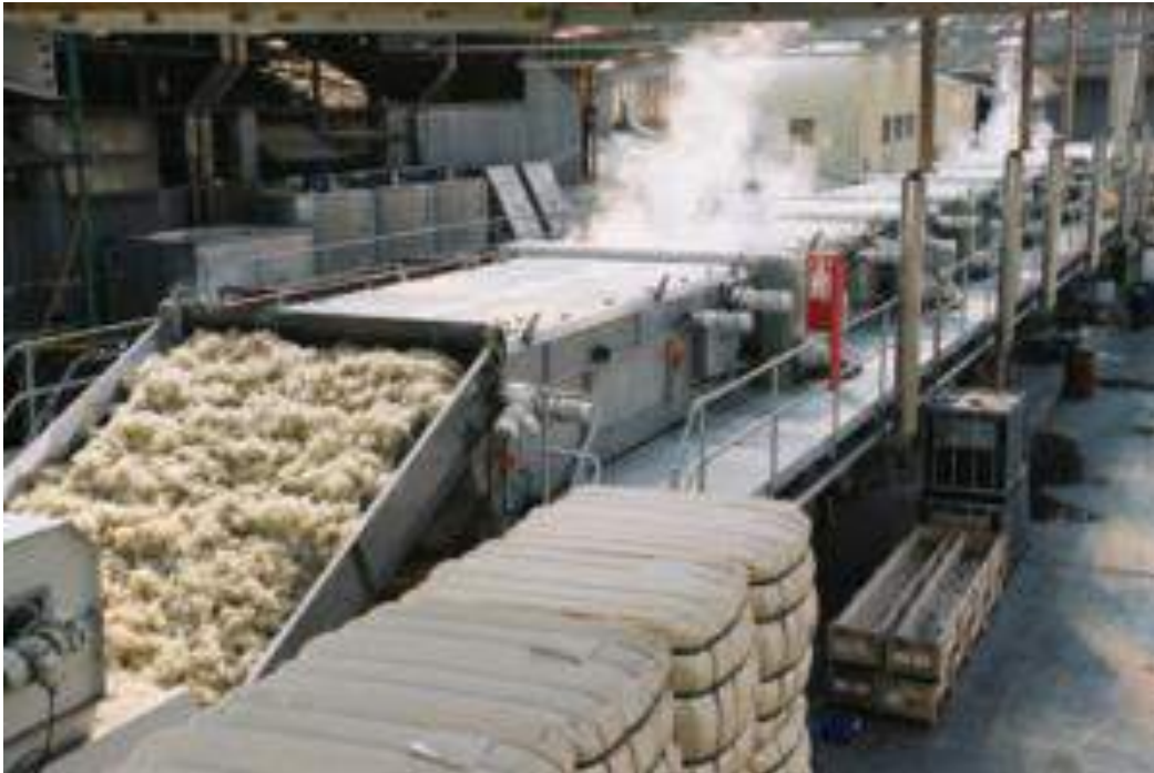
Photo: Wool fibre scouring Plant
