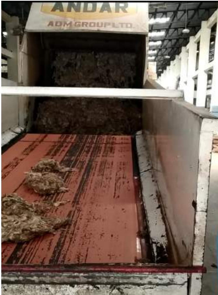
Photo: Feeding of raw wool (wool fibre scouring machine)
