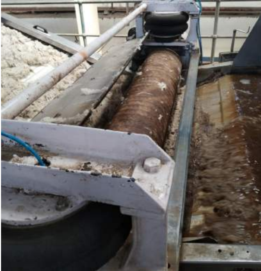
Photo: wool fibre scouring (after scouring in first Bowl the fibres are squeezed and forwardd to second Bowl)
