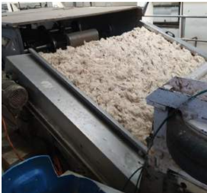
Photo: wool fibre scouring (after scouring in first Bowl the fibres are squeezed and forwardwd to second Bowl)
