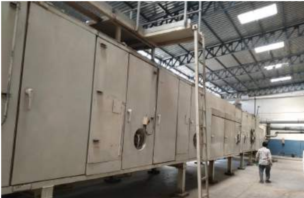
Photo: Wool fibres drying machine (1)
