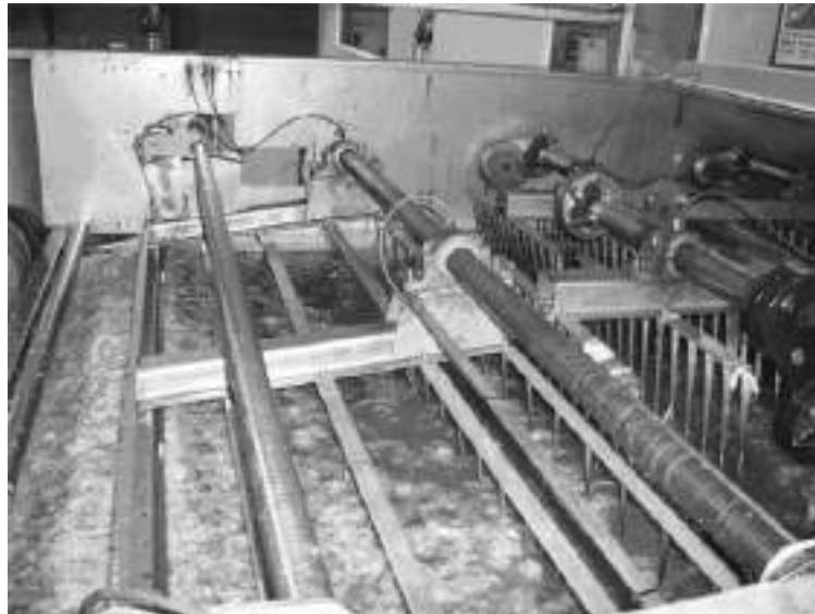
Figure: Immersed wool being moved by the rakes in a scouring bowl.
