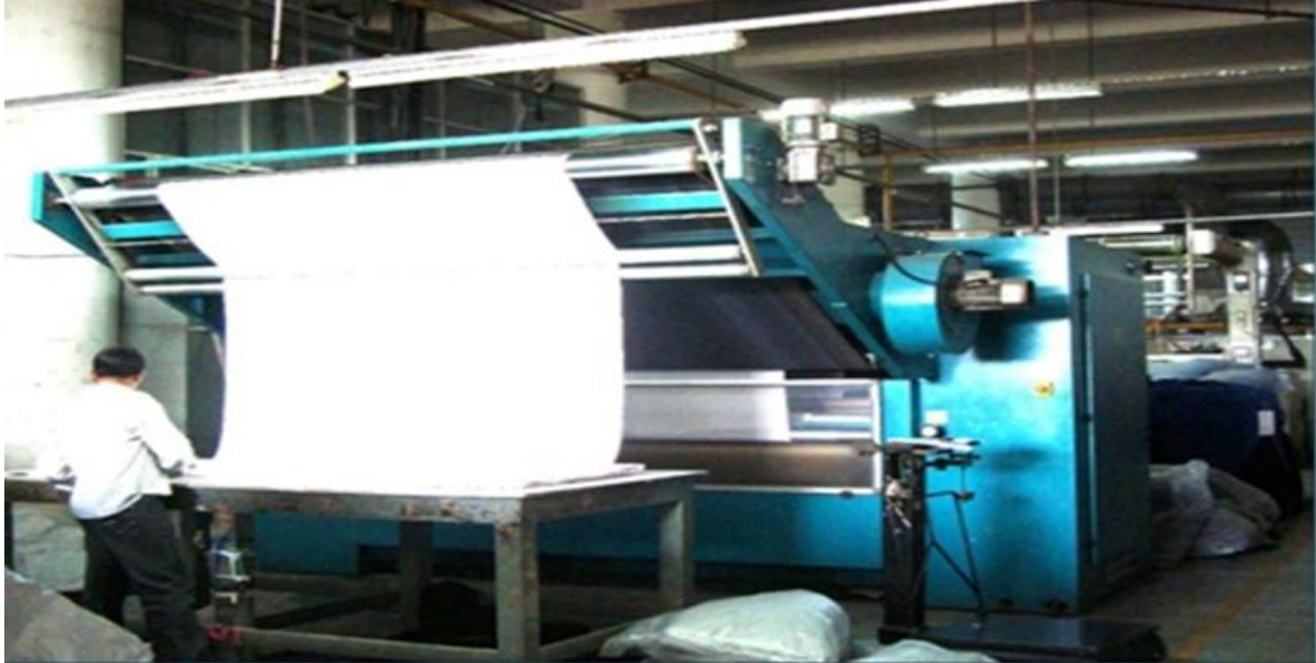
Operator observing defects at the exit unit
