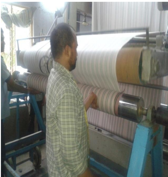
Setting empty batch for winding
