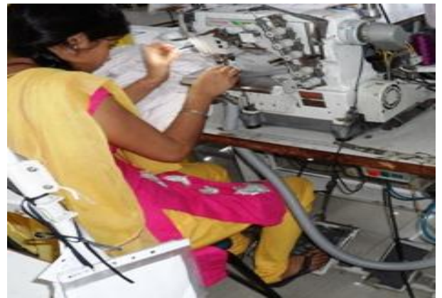
Threading on Flatlock machine Step 4
