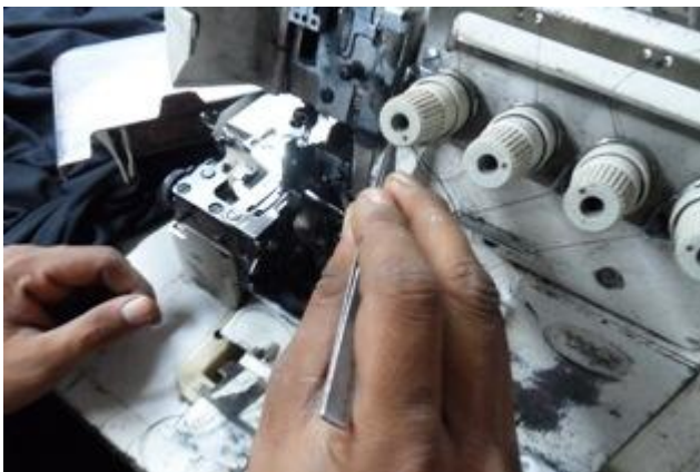
Threading on Overlock machine Step 3
