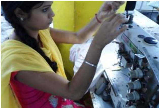
Threading on Flatlock machine Step 3
