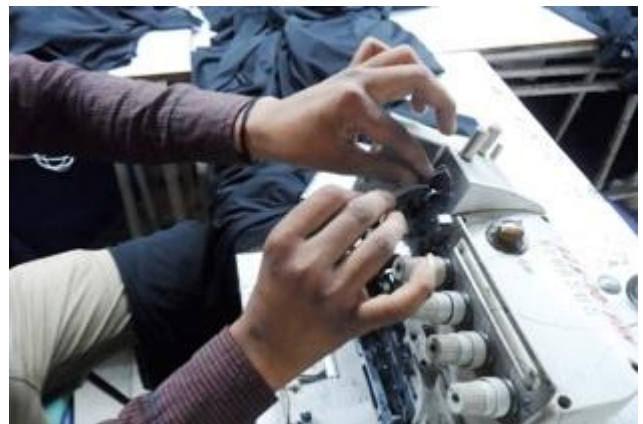
Threading on Overlock machine Step 4
