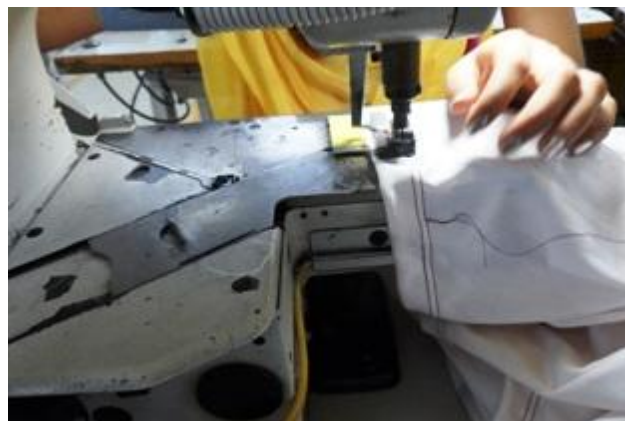
Start Stitching on Flat lock Machine
