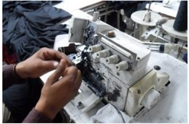
Threading on Overlock machine Step 2
