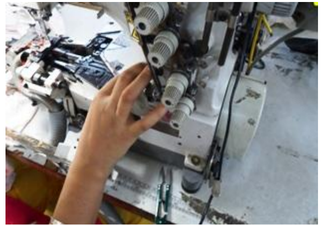
Threading on Flatlock machine Step 2
