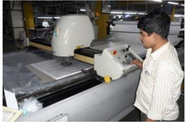
Cutting operation by Computerized cutting machine
