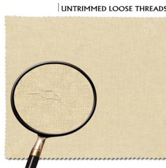
UNTRIMMED LOOSE THREADS
