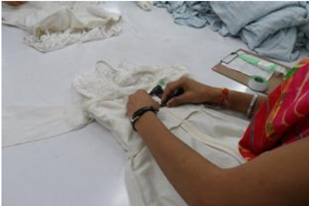
Removing loose threads
